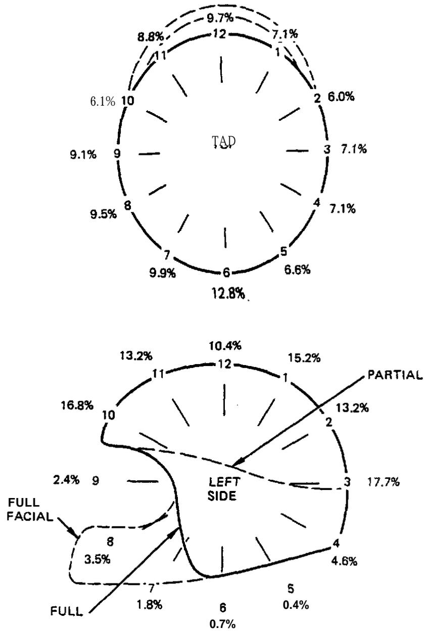
Table 9.8.13 (Appendix c.5) shows the **measured** liner crush, or **compression** permanent deformation, **at** the **two** most severe impact points on the motorcycle rider helmet. **Because** of the variation of recovery of the many different liner **materials**, it **was** difficult to relate this single measurement to **impact severity**. Only the **styrofoam** liner with low recovery gave consistent indications of impact severity.
